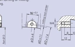
**Inclined milling tool HSS** ld. No. 033611
