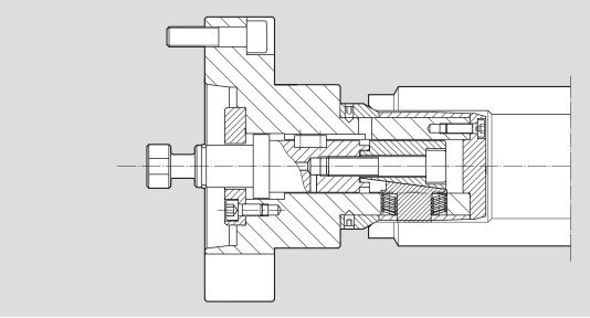
**Example:** Special expanding mandrel, double taper design with retractable stop, for clamping of stators
