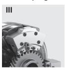
Optionally prelocator pins are available. Prelocator pins are used at automatic loading. The determination is made according to the clamping pins used.
