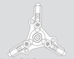
Determination of height of locator posts:  $\Delta$  = Distance between clamping position and locating face Height of locator posts [H] = 32.5 mm -  $\Delta$
