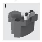
At first you need to choose your matching top jaw (size 1 - 6) for the outside diameter [da] of the gear to be machined. Each size of top jaw can cover 20 mm outside diameter using two different types of clamping pins (Type A and B). One set of top jaw consists of 3 pieces including 1 straight key
